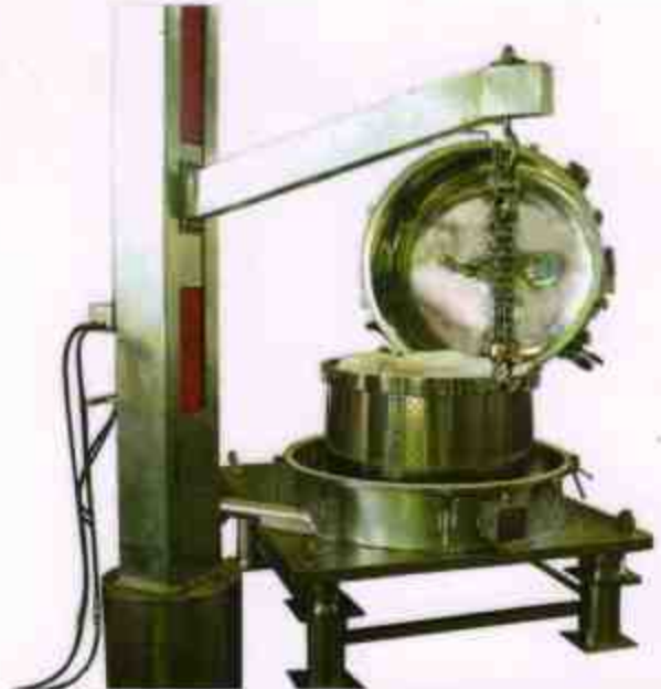
DOME OPEN LIFTING BAG TYPE MACHINE WITH LIFTER FOR EASY REMOVAL OF MATERIAL
